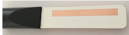
Sensor surface after exposure. Tarnish was completely dissolved by the grease.
